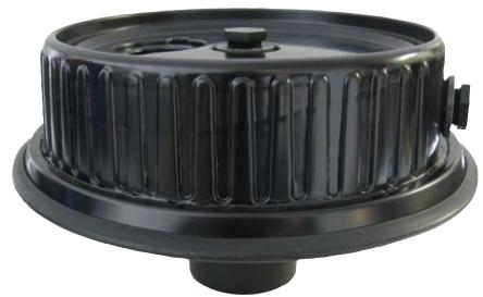
Install the lower half of the bottom drain at the predetermined point in your pond, attaching it to the PVC elbow pipe with PVC glue. It is important that this connection is totally secure. When this step is complete, the installed piece should be recessed at least 3/4" below the level of the pond bottom.
