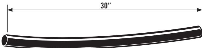
2. If using a Snorkel™ Vault Extension, an additional length of 2" Flex PVC will be required.
