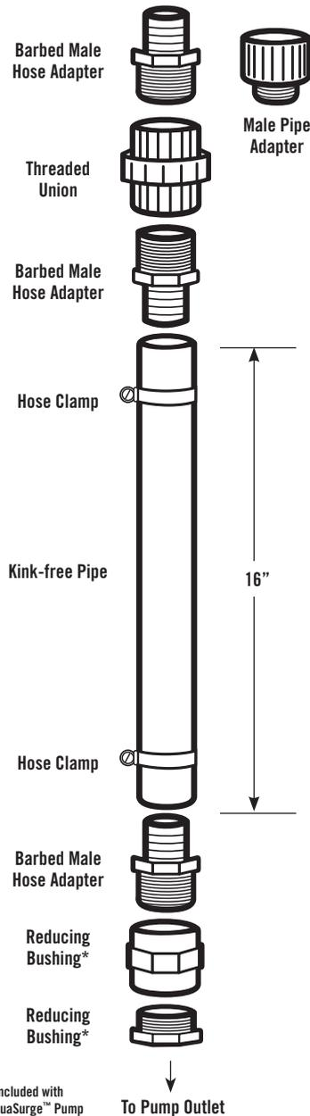
**NOTE:** You can either use the male pipe adapter (flex PVC) OR the 1 1/4" x 1 1/2" barbed male hose adapter (kink free) that threads into the union.
