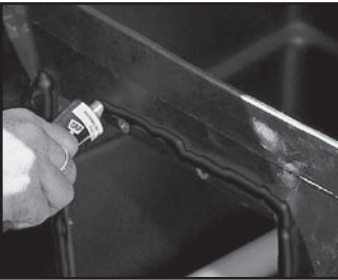
Fig. 13 Apply a bead of fish-safe silicone sealant around the skimmer opening, over the nut inserts.
