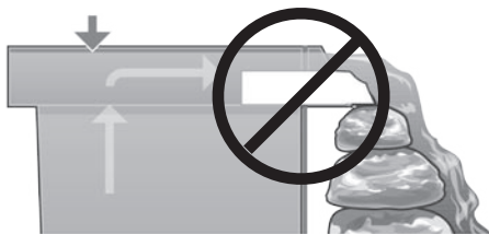
Fig. 12 If a thick rock along with a larger flow pump is used, the water flow may be so great that it will flow over the sides of the BIOFALLS® filter.
