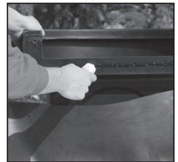
Fig. 8 Remove waterfall lip and apply a thick bead of fish-safe silicone sealant around the MicroFalls® filter opening.
