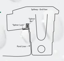
sible. The liner should be run up the stream or to the filter box. Folder the liner over the Spliner Lock. Slide the Spliner Bar into the spline channel and secure with the Spliner Locks. Be
