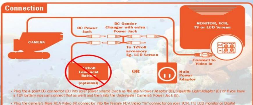
• The second DC power plugican be connected to your 12V Viewing Device, such as a portable LCD screen.
