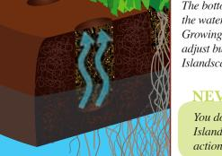
The bottom of the wicking channels must be in contact with the water so that wicking action can occur. Confirm that the Growing Media is appropriately moist after launch. You can adjust buoyancy by adding or subtracting rocks to the top of the
