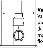
Valve open Valve at 90° position (left/right) maximum flow
