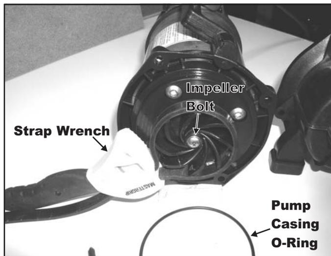
2. Remove the pump casing o-ring. Hold the impeller with a strap wrench and remove the impeller bolt.
