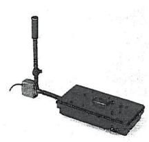
CARE AND INSTRUCTIONS: THE POND FILTER RESTS ON THE BOTTOM AND IS DESIGNED TO CONNECT TO THE INTAKE OF A SUBMERGED PUMP BY THE 1" ID TUBING INCLUDED. IN LARGER PONDS, A LONGER PIECE OF TUBING CAN BE USED SO THAT THE FILTER CAN BE MOVED AS NEEDED TO COLLECT DEBRIS WHILE THE PUMP REMAINS STATIONARY. TWO OR MORE POND FILTERS MAY BE "TEE'D" TOGETHER FOR LARGER PONDS AND PUMPS.
