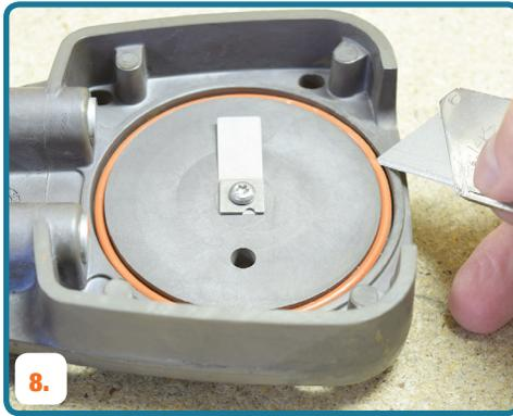
**8.** Remove the cylinder o-ring(s) from the bottom of valve plate(s) and install new o-rings.
