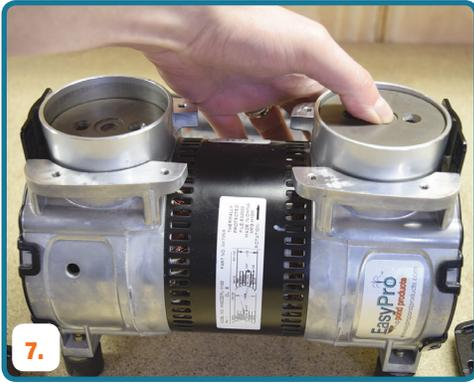
**7.** Press retainer plate with piston cup into cylinder all the way to the piston. The cylinder can be rotated to align the screw holes. Apply thread locking compound (Loctite® 222) to retainer screws, torque screws to 10-13 inch-pounds.
