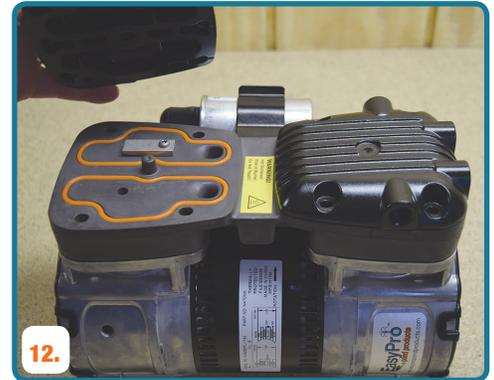
**12.** Reinstall head over valve plate(s) checking that orientation with ports is correct. Torque screws to 50 inch-pounds
