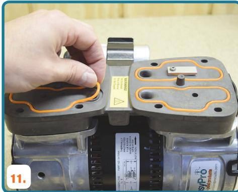
**11.** Remove old and install new head o-rings in the o-ring grooves on top of valve plate
