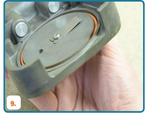
**9.** Inspect the leaf valves for damage or wear. NOTE: There is one intentionally “bent” leaf valve per set. If leaf valves need to be replaced, a complete leaf valve plate can be ordered. The screws holding the leaf valves are susceptible to breaking which makes individual leaf valve replacement very difficult.
