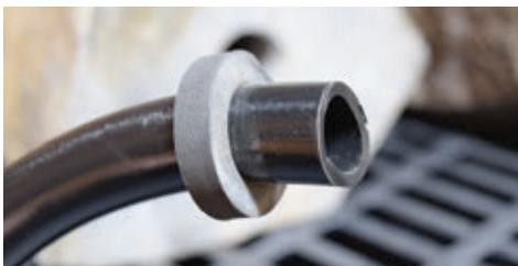
**4** Carefully press the assembled friction ring (4A) and tubing into the bottom hole of the basalt. It will be a very tight fit. The use of a dull object (i.e. unsharpened pencil) can be used to help press the friction ring into the hole. (4B) Press until friction ring is below the surface of the basalt. (4C) Avoid breaking or tearing the friction ring or water will not travel properly up the column.
