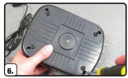
Re-install screws into compressor housing.
