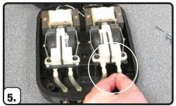
Match the air outlets to the air tubes and re-install screws.
