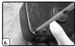
Re-install screws into compressor housing.
