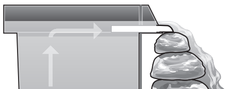
Fig. 35 If using a natural rock for your waterfall weir, make sure that it is fairly thin. (no more than 3/4")
