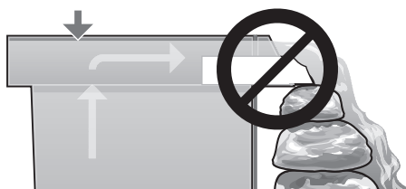
Fig. 36 If a thick rock along with a larger flow pump is used, the water flow may be so great that it will flow over the sides of the UltraFalls™.
