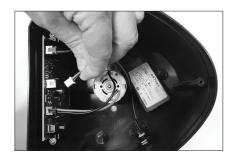
7. Fit battery plug into socket on PCB board.
