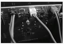
8. Battery plug should be fitted as shown above.
