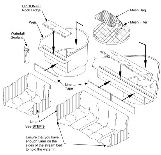
STEP 7: You can either cut a piece of liner the width of your Waterfall Weir (24" wide or 40") or pull your existing liner from your pond and attach it to the Liner Tape.
