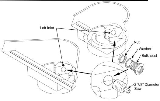
STEP 1: Decide the location of the Weir keeping in mind that the Waterfall generally faces the viewing area. Ensure you have enough dirt for a sloping stream bed that drains into the Pond. Choosing the Left or Right Inlet Installation should be decided at this point.
