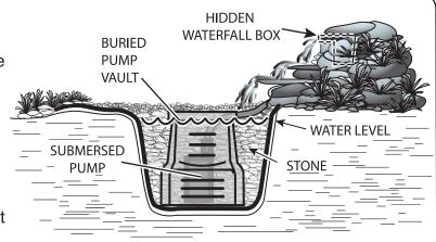
service. Your Pump Vault is designed to allow one or more pumps to be placed deep down in the gravel bed and still be easily accessible. In addition, your Pump Vault can be fitted with an optional automatic fill valve to keep the water level in the gravel bed at an optimal level.
