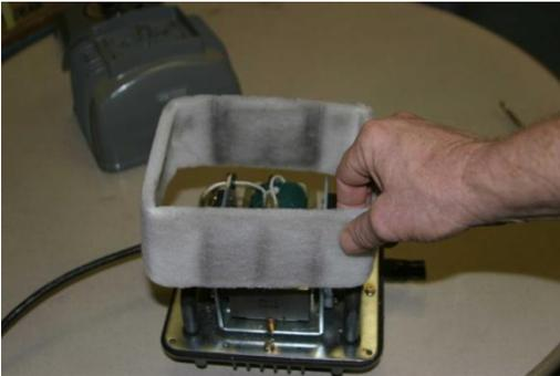
16) Replace the outer metal housing onto the base and tighten the 4 screws. Wash the square air filter with tap water and shake dry. Reinstall into the top of metal housing and replace the filter cover. Congratulations, you've done it!
