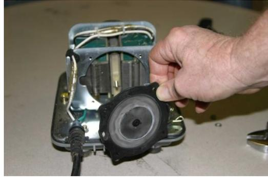
\*At this point you will have a better look at the magnet. The magnet rarely needs to be replaced. If there is a lot of fine metal dust in the motor area then the magnet may need to be replaced. Inspect the top and bottom part of the magnet. If it looks very worn or melted proceed to the optional section on "How to Replace the Magnet".
