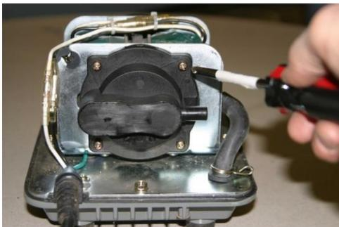
14) Replace the black J-Tube over the diaphragm outlet. Use existing clip to secure tube to outlet.
